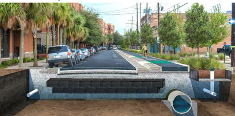
Figure SW-5: Rendering of Baronne Street with Subsurface Storage Tanks (Image Credit: Dana Brown & Associates)
